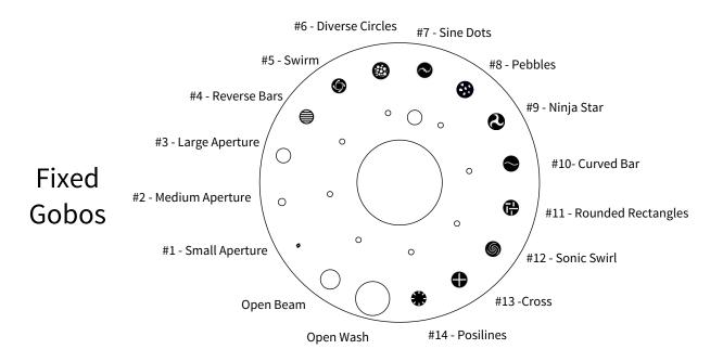
NOTE: All fixed gobos oriented as projected from fixture, not stamped orientation
