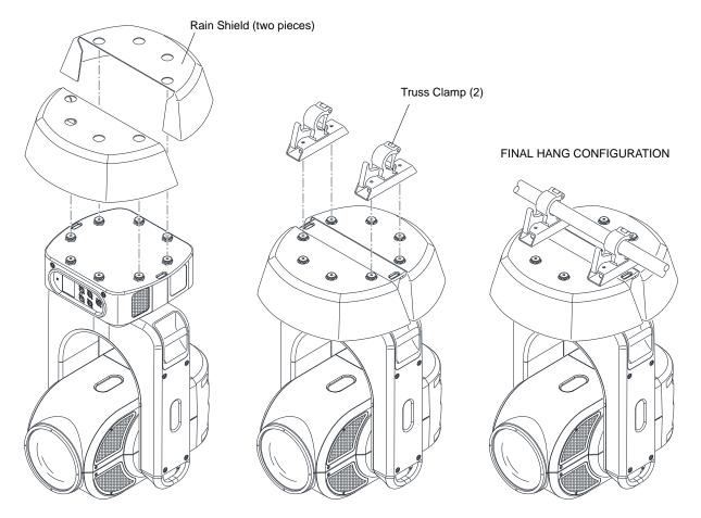
Figure 2: Installing Hanging Rain Shield 1
