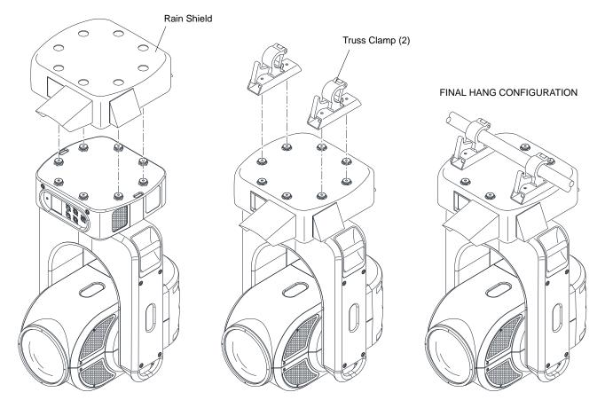
Figure 3: Installing Hanging Rain Shield 2
