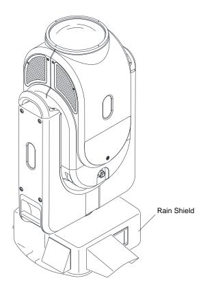
Figure 4: Installing Floor Standing Rain Shield
