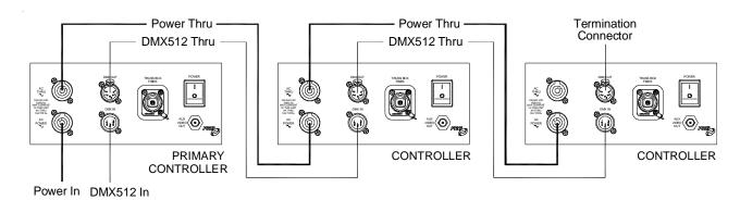
Figure 3: Example Daisy-Chain Configuration
