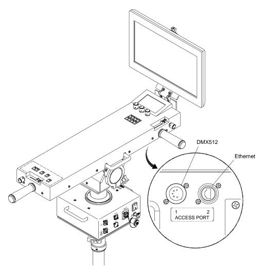
Figure 2: Access Ports
