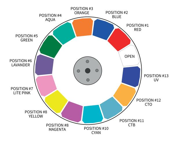
The following charts represent the fixed color wheel configurations for the ICON Beam luminaire.
