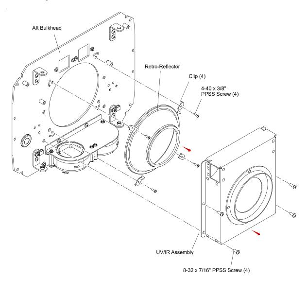
Figure 3-48: Replacing Retro-Reflector
