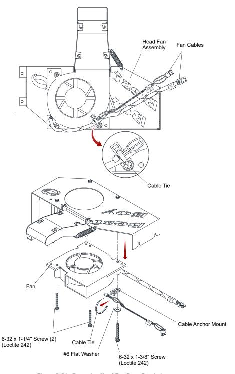
Figure 3-21: Removing Head Fan From Bracket
