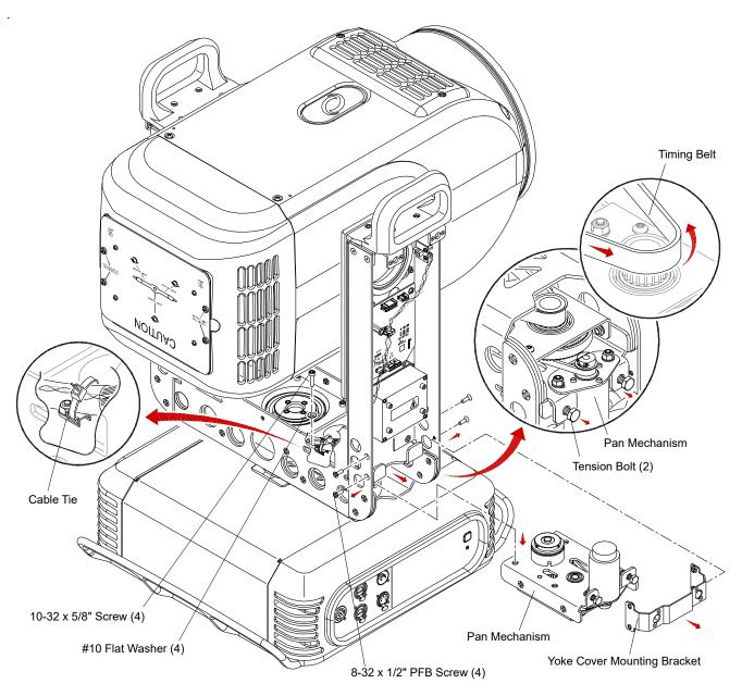
Figure 3-63: Removing Pan Drive Mechanism
