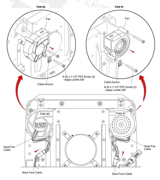
Figure 3-42: Replacing Back Fan #1 or #2
