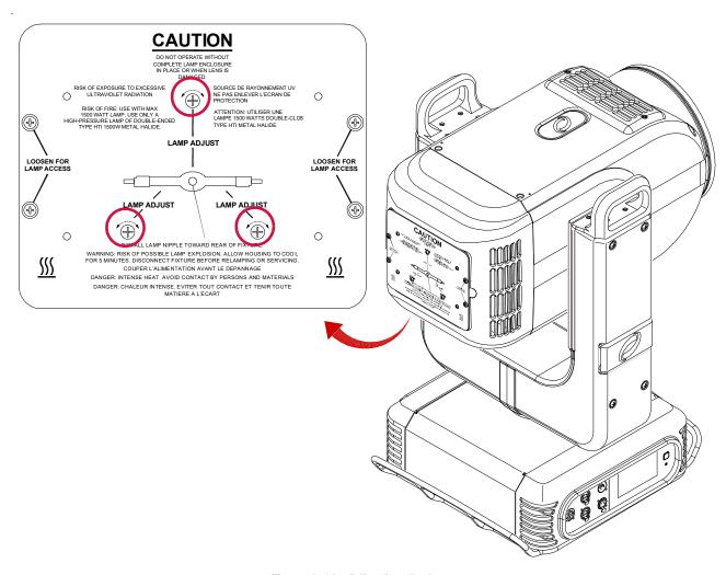
Figure 3-10: Adjusting the Lamp
