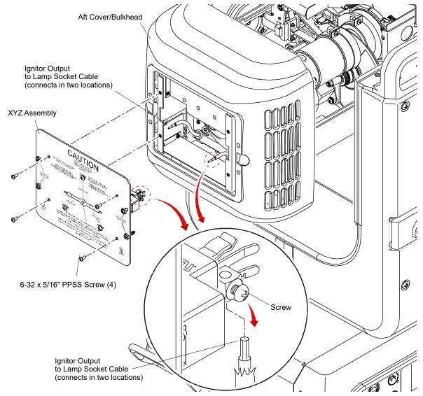
Figure 3-3: Removing XYZ Assembly
