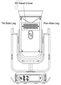
Figure 1-3: Yoke Leg Identification
