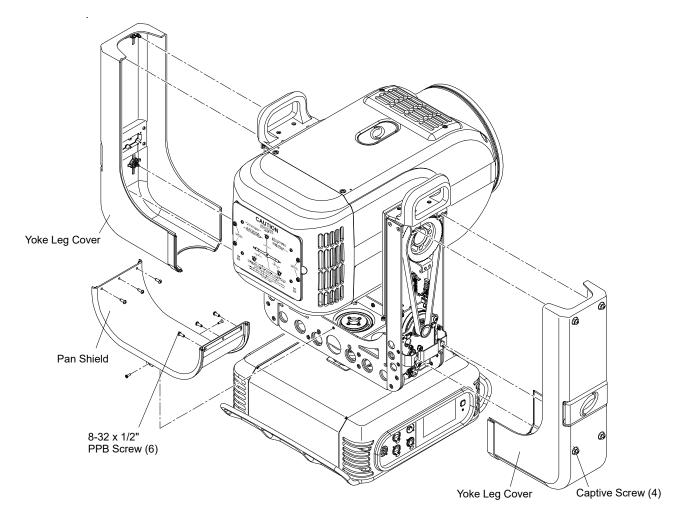
Figure 3-58: Removing Yoke Leg Covers and Pan Shield
