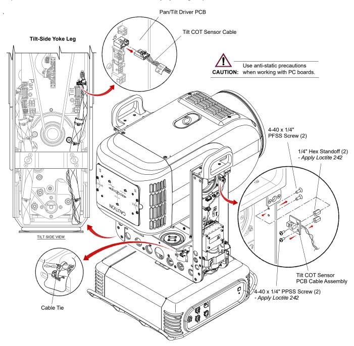
Figure 3-59: Removing Tilt COT Sensor PCB
