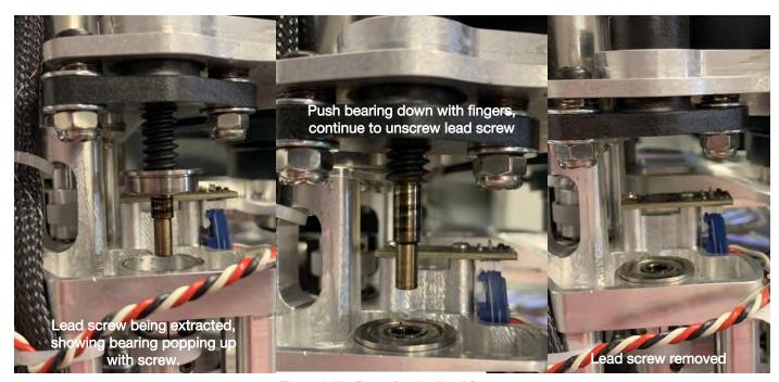
Figure 3-40: Removing the Lead Screw
