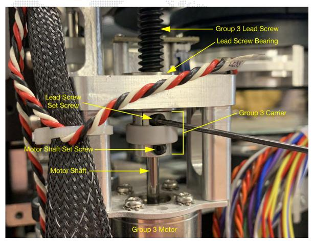
Figure 3-39: Group 3 Lens Motor Assembly Detail
