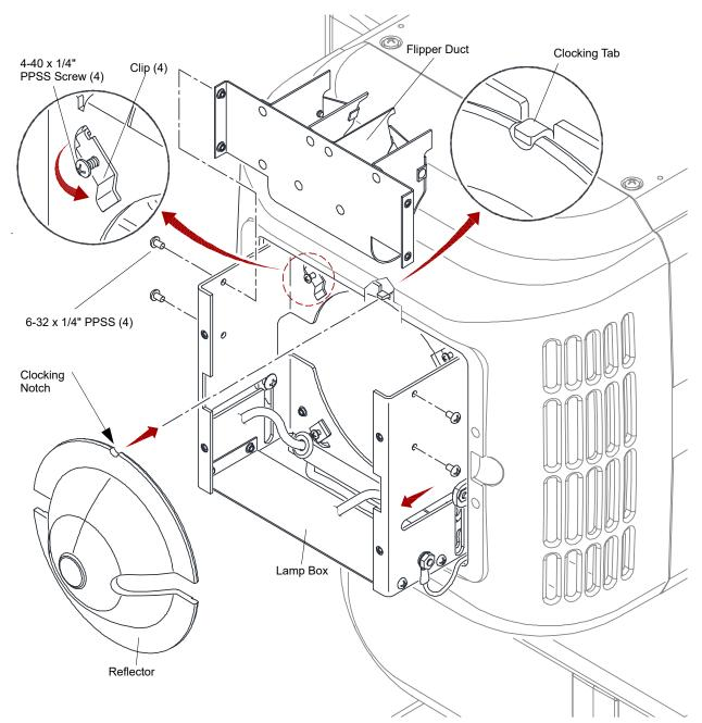
Figure 3-46: Replacing Reflector
