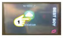
Bypassing CALIBRATION on Startup
