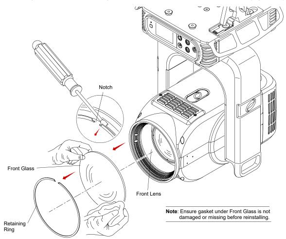
Figure 3-8: Removing Front Glass
