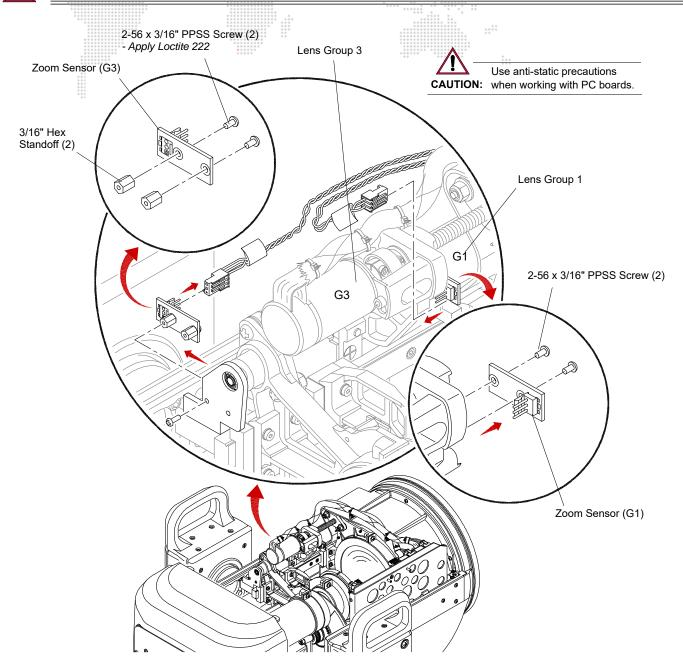
Figure 3-31: Removing Zoom Sensors 1 & 3
