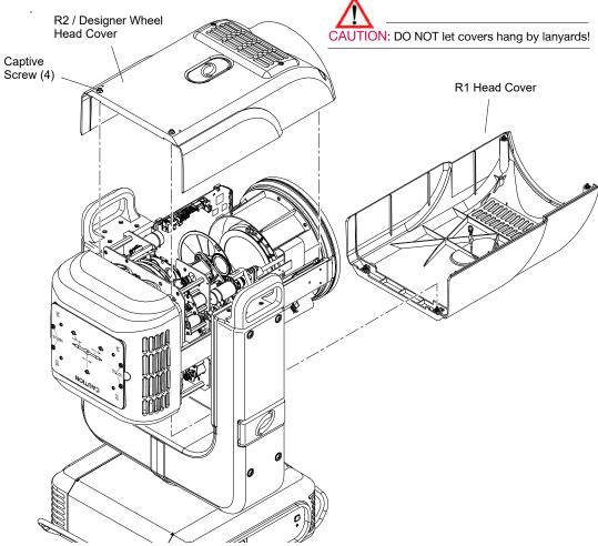
Figure 3-2: Removing Head Covers
