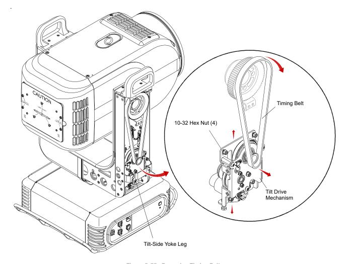
Figure 3-56: Removing Timing Belt
