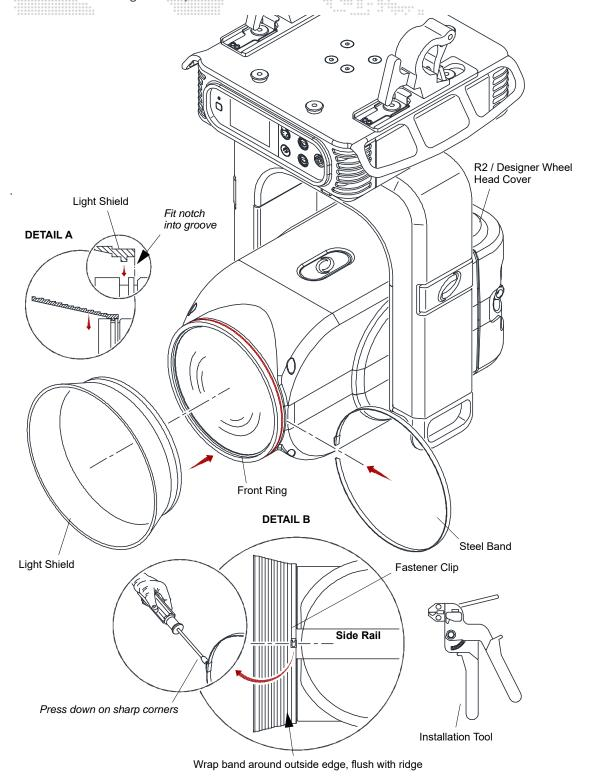
Figure 3-19: Installing Light Shield with Steel Band
