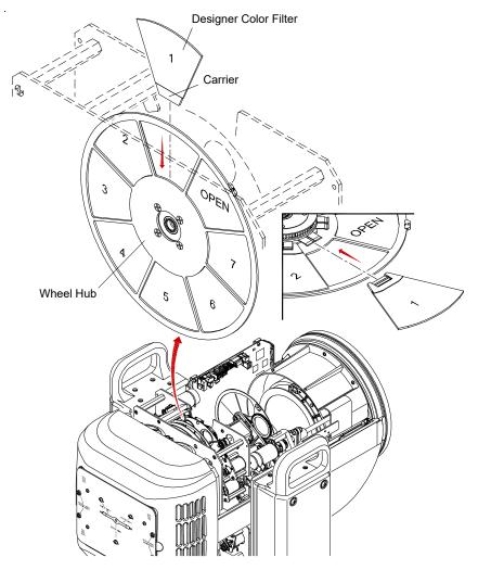
Figure 3-16: Removing a Designer Color Filter
