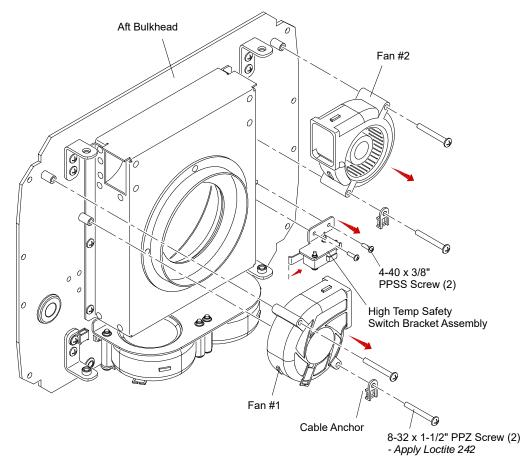
Figure 3-47: Removing Fans and HIgh Temp Safety Switch
