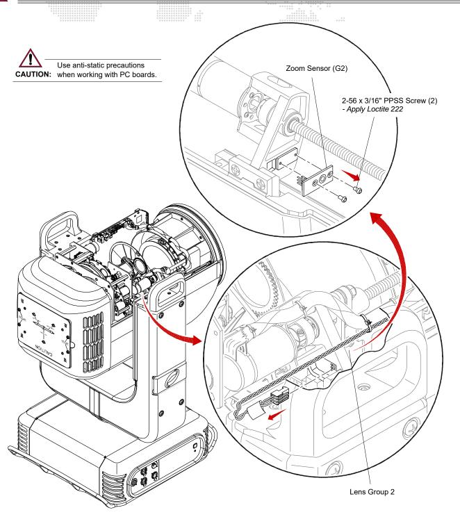
Figure 3-32: Removing Zoom Sensor 2
