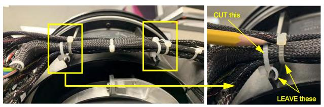
Figure 3-37: Freeing Cable Bundles from Group 3 Light Shield
