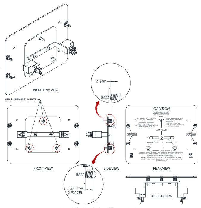
Figure 3-11: Measuring Lamp Alignment Position
