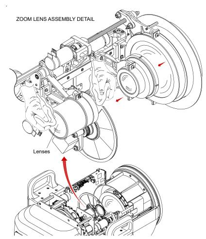
Figure 3-7: Accessing Zoom Lens Assembly
