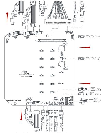
Figure 3-22: Head Controller PCB Cable Connections
