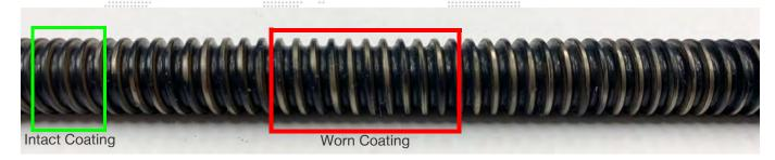
Figure 3-36: Lead Screw with Coating Worn from Threads
