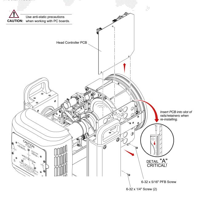
Figure 3-23: Removing Head Controller PCB
