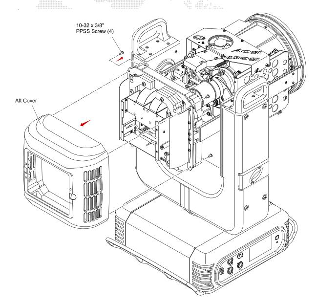
Figure 3-4: Removing Aft Cover
