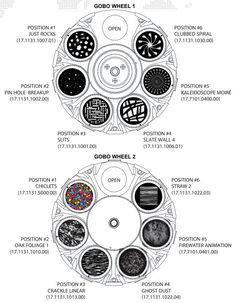
Figure 1-8: Gobo Wheel Standard Configurations
