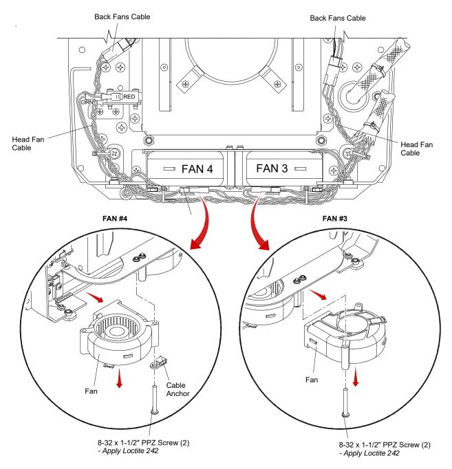
Figure 3-43: Replacing Back Fan #3 or #4
