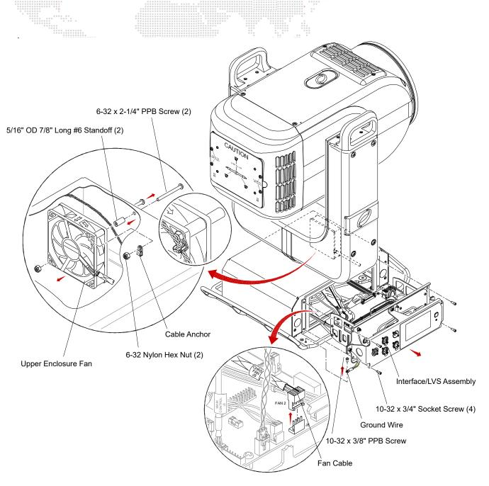
Figure 3-53: Removing Upper Enclosure Fan
