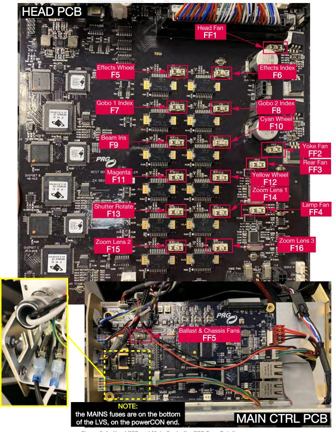
Figure 2-4: Head PCB and Main Controller PCB Fuse Detail
