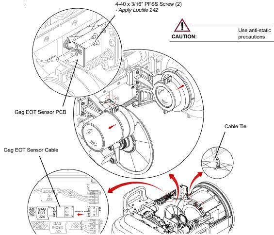
Figure 3-28: Removing Gag Sensor Cable Assembly
