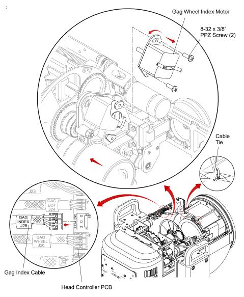
Figure 3-30: Removing Gag Wheel Index Motor
