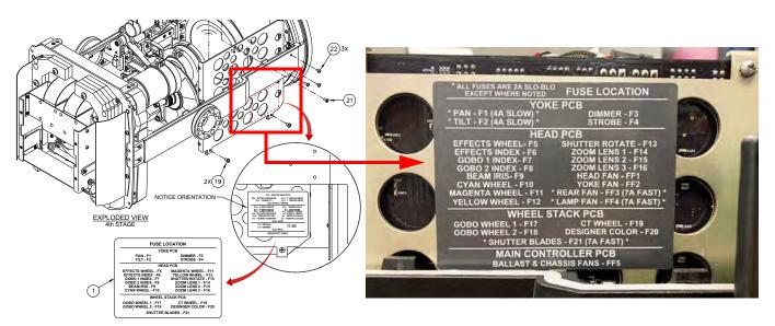
Figure 2-2: Fuse Map Location on Head PCB Bracket
