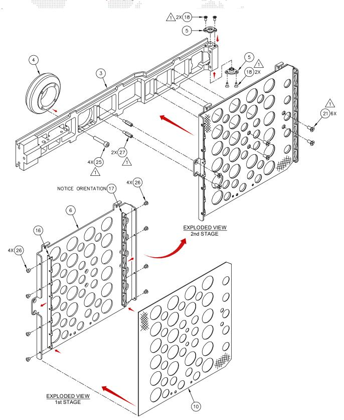
**Head Assembly (continued)** Refer to Parts List for "Head Assembly" on page 153. ASSEMBLED ISO VIEW SIDE RAIL & BRACKET EXPLODED VIEW 3rd STAGE
