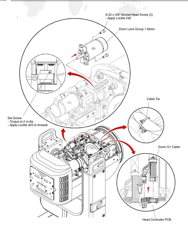
Figure 3-33: Removing Zoom Lens Group 1 Motor
