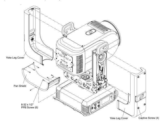
Figure 3-62: Removing Yoke Leg Covers and Pan Shield
