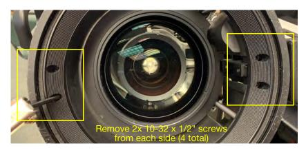
Figure 3-38: Removing the Light Shield Assembly
