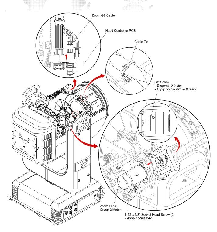
Figure 3-34: Removing Zoom Lens Group 2 Motor
