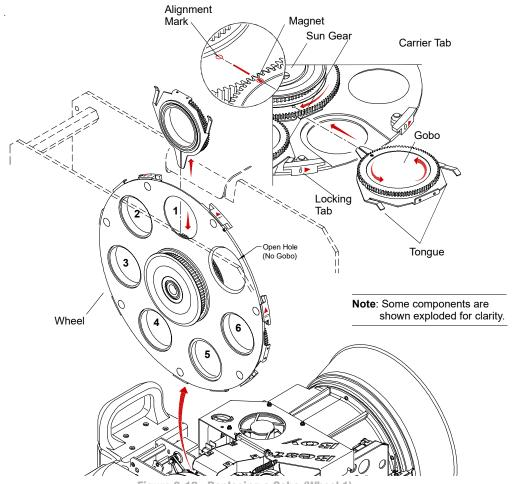
Figure 3-12: Replacing a Gobo (Wheel 1)
