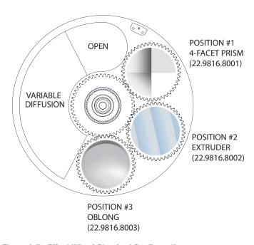
Figure 1-7: Effect Wheel Standard Configuration
