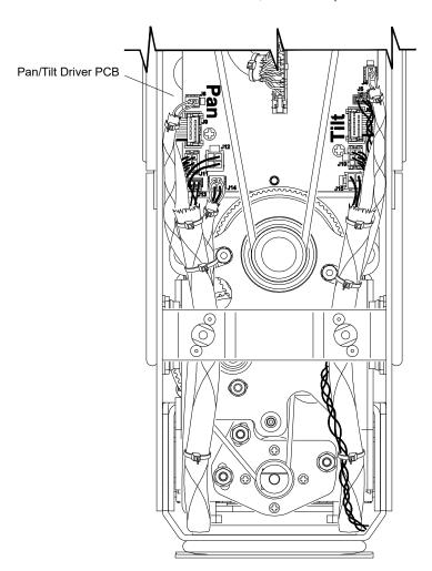
Figure 3-60: Tilt-Side Yoke Leg with Pan/Tilt Driver PCB
