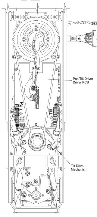
Figure 1-4: Tilt-Side Yoke Leg
