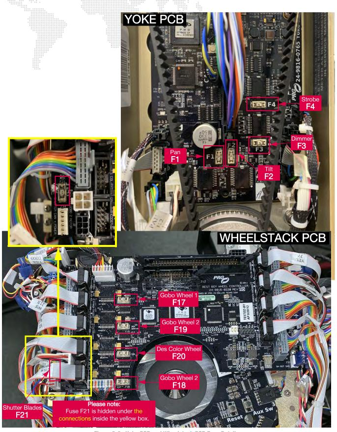
Figure 2-3: Yoke PCB and Wheelstack PCB Fuse Detail
