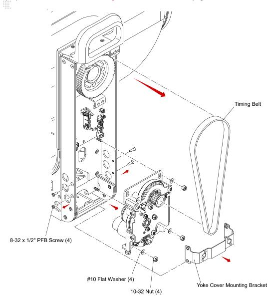
Figure 3-61: Removing Tilt Mechanism
