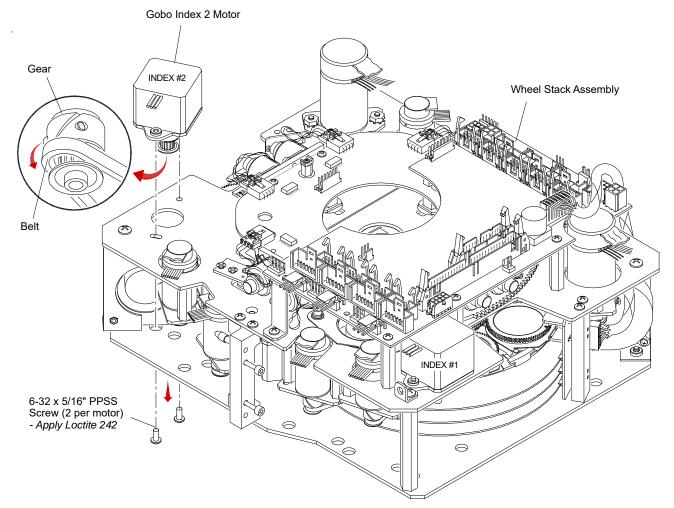
Figure 3-27: Removing Gobo Index 2 Motor
