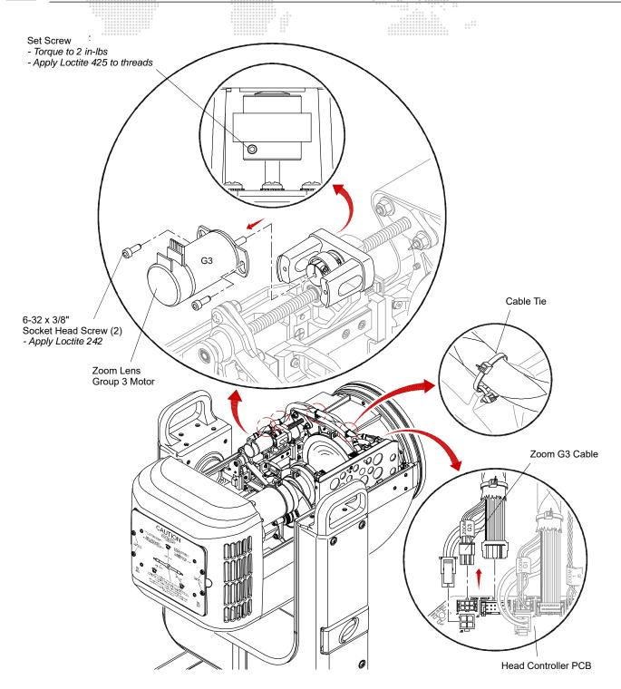
Figure 3-35: Removing Zoom Lens Group 3 Motor
