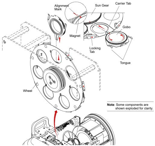
Figure 3-14: Replacing a Gobo (Wheel 2)
