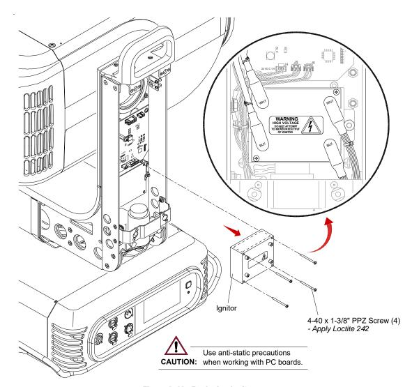
Figure 3-49: Replacing Ignitor
