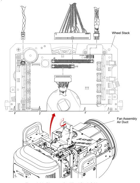
Figure 3-24: Disconnecting Wheel Stack Cables
