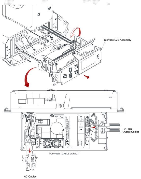
Figure 3-52: Removing Interface/LVS Assembly
