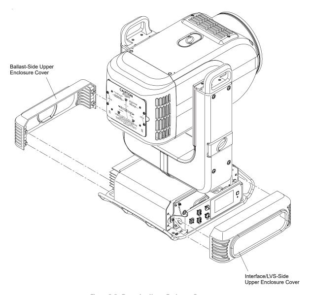
**Figure 3-6: Removing Upper Enclosure Covers**
