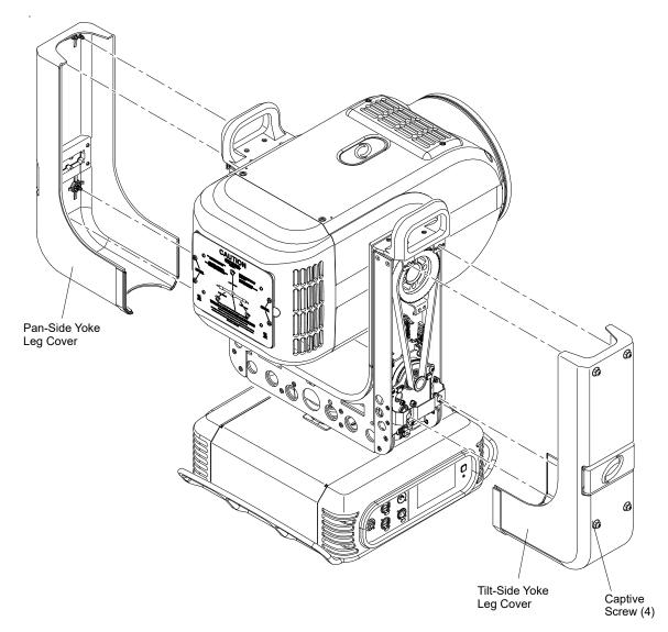
Figure 3-5: Removing Yoke Leg Covers
