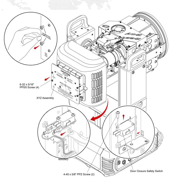
Figure 3-44: Replacing Door Closure Safety Switch
