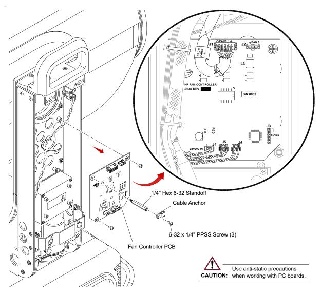
Figure 3-50: Replacing Fan Controller PCB
