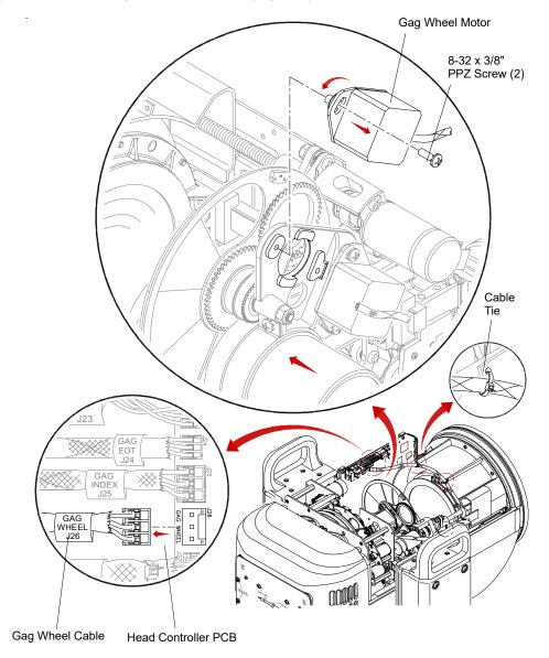
Figure 3-29: Removing Gag Wheel Motor
