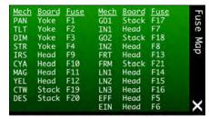
**Fuse Map** - Provides the circuit board location for all mechanism fuses.
