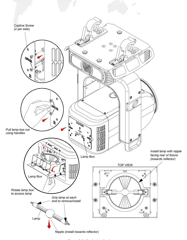
Figure 3-9: Replacing the Lamp
