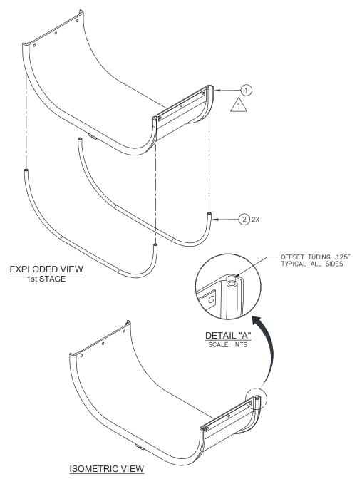
CLEAN W/PERMA BOND POP POLYOLEFIN PRIMER BEFORE APPLYING PERMA BOND 737 CYANOACRYLATE THEN APPLY ADHESIVE DIRECTLY TO PLASTIC SURFACE. DO NOT STRETCH TUBING WHEN INSTALLING.
