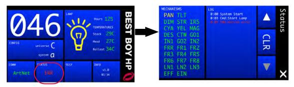
The Status screen will indicate which specific mechanisms, if any, have errors. It also provides a log of systems activity. The Status screen operates as follows:
