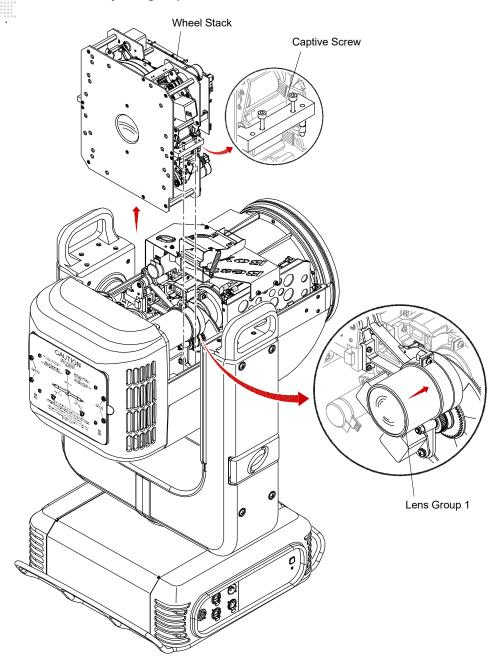
Figure 3-25: Removing Wheel Stack
