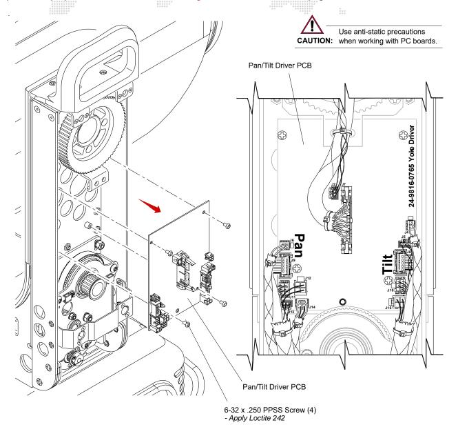
Figure 3-57: Removing Pan/Tile Driver PCB
