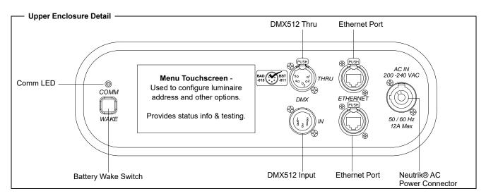
Figure 1-1: Exterior Components
