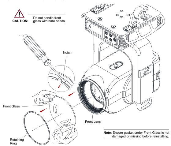
Figure 3-18: Removing Front Glass
