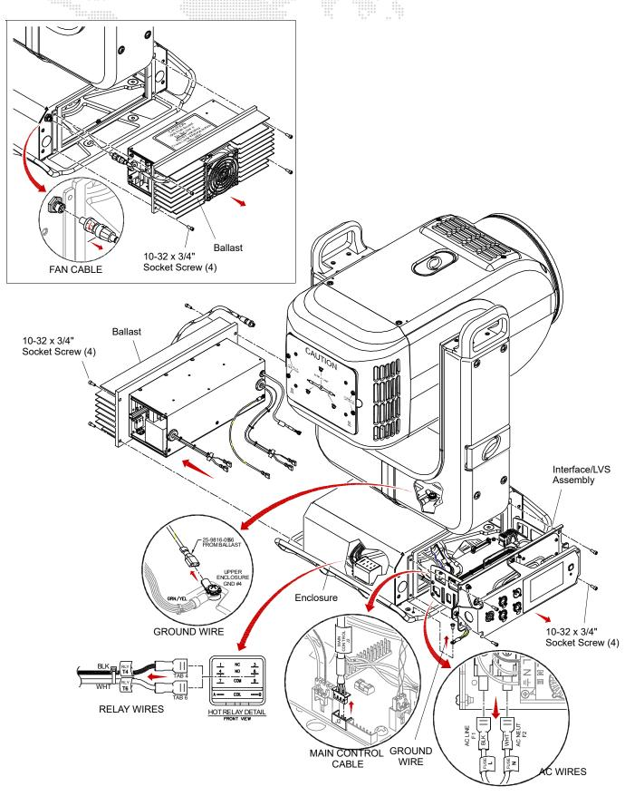
Figure 3-54: Removing Ballast
