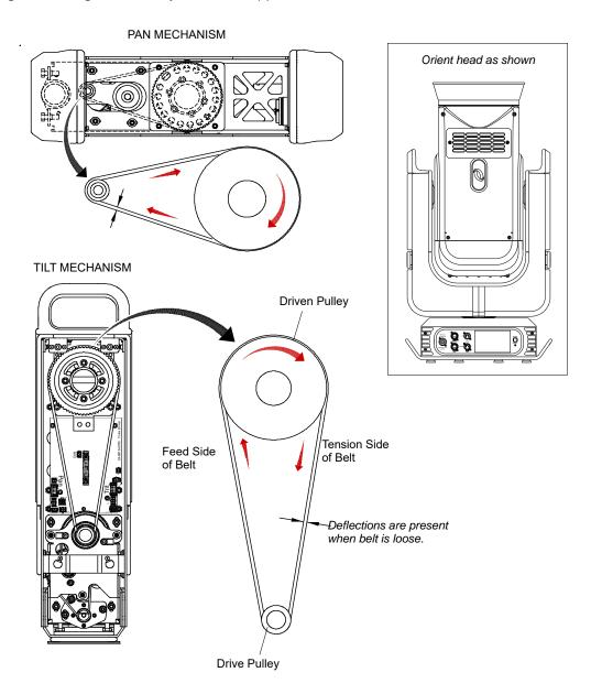
Figure 3-64: Belt Tension Adjustment
