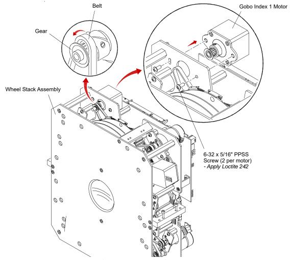
Figure 3-26: Removing Gobo Index 1 Motor
