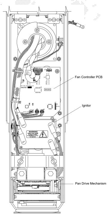
Figure 1-5: Pan-Side Yoke Leg
