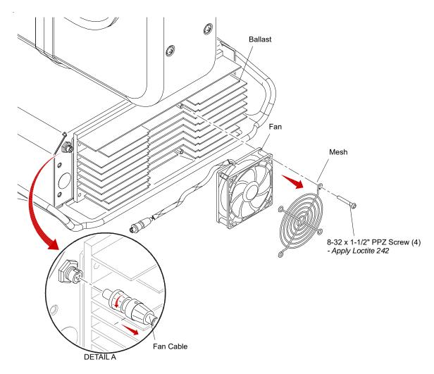
Figure 3-55: Removing Ballast Fan
