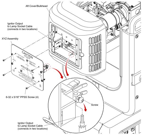
Figure 3-45: Removing XYZ Assembly
