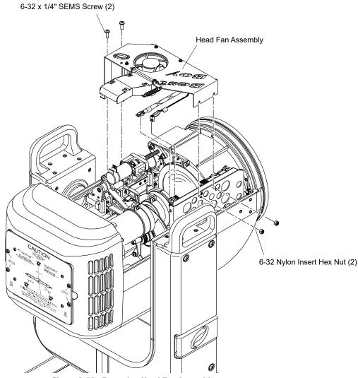
Figure 3-20: Removing Head Fan Assembly
