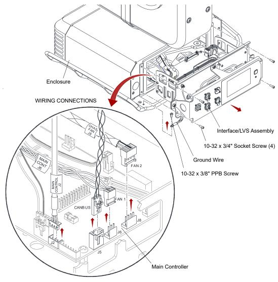
Figure 3-51: Disconnecting Interface/LVS Cables
